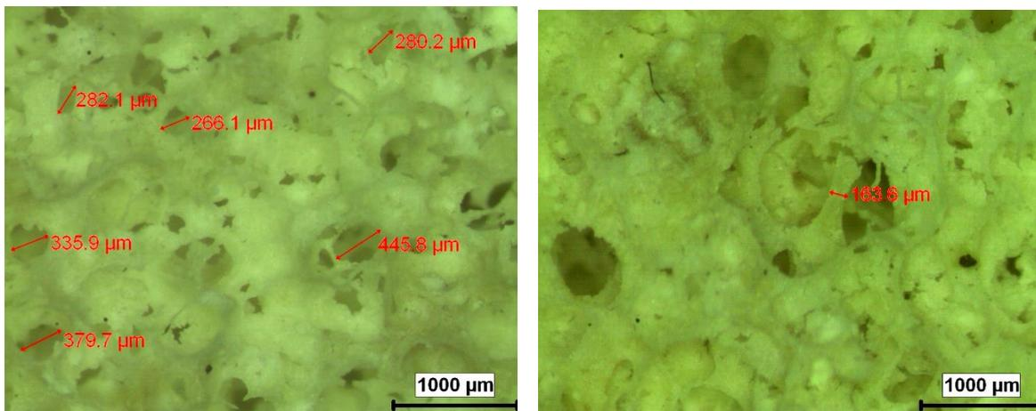
Figure 9. Pore size and arm thickness in the HA samples with 10% bentonite
