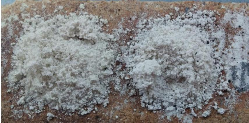
Figure 2. The collapsed HAp foams
