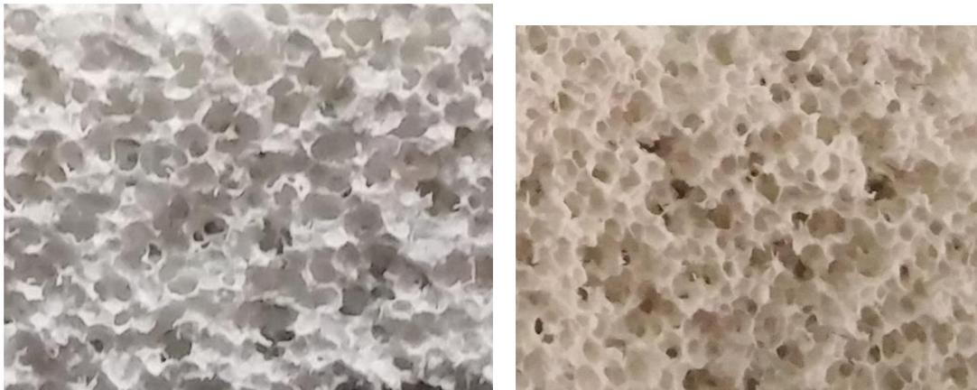
Figure 3. The reticulated structures of HAp prepared from a) finer powder b) coarser powder
