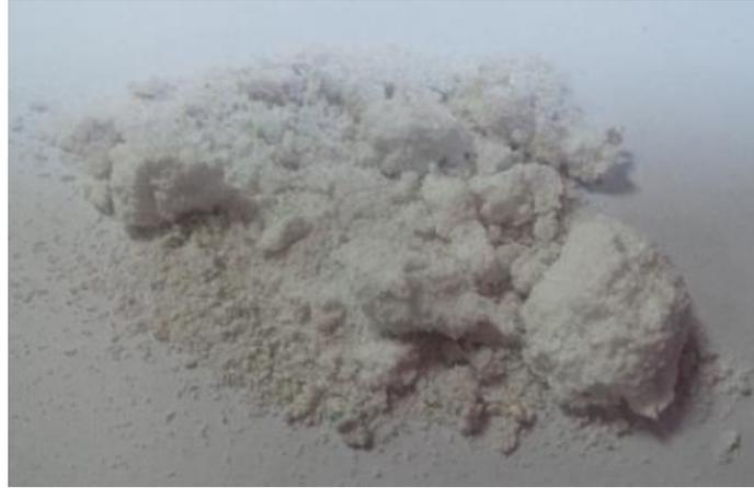
Figure 4. The collapsed HA foam produced from spray dried powder after sintering
