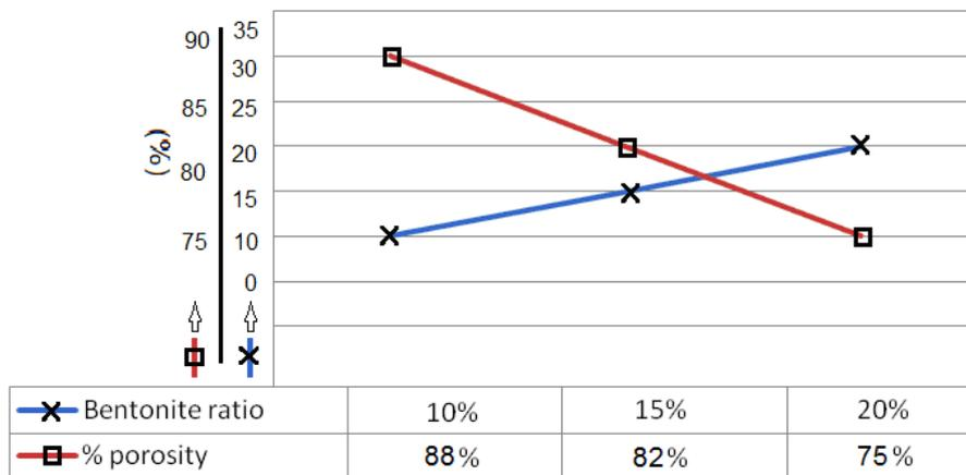
Figure 8. The relation of porosity and bentonite rate
