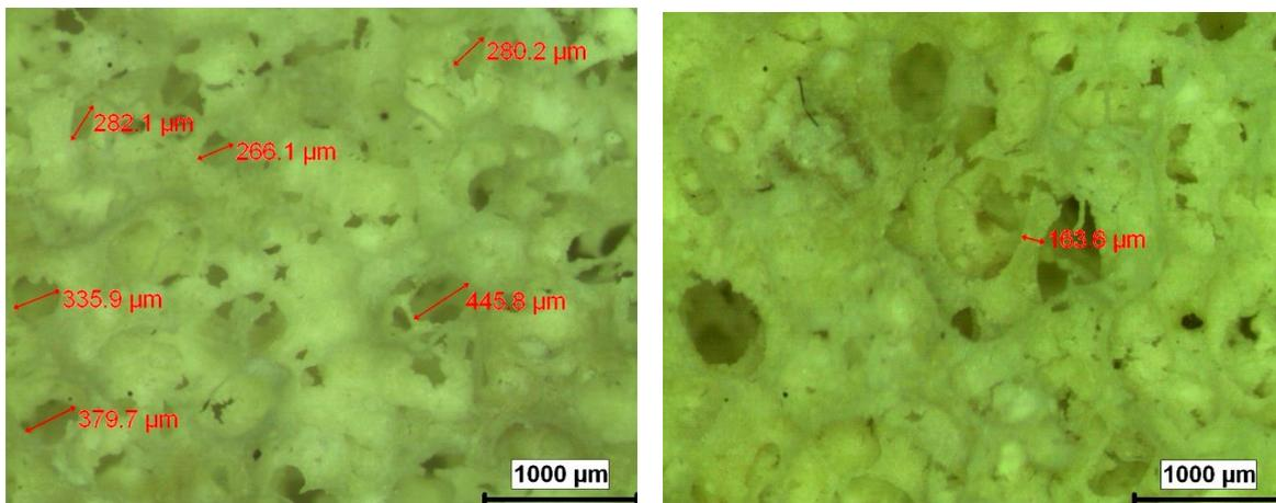
Figure 9. Pore size and arm thickness in the HA samples with 10% bentonite
