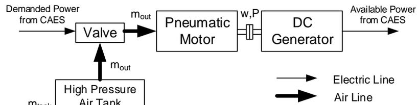
Figure 1. Block diagram of the CAES system.
