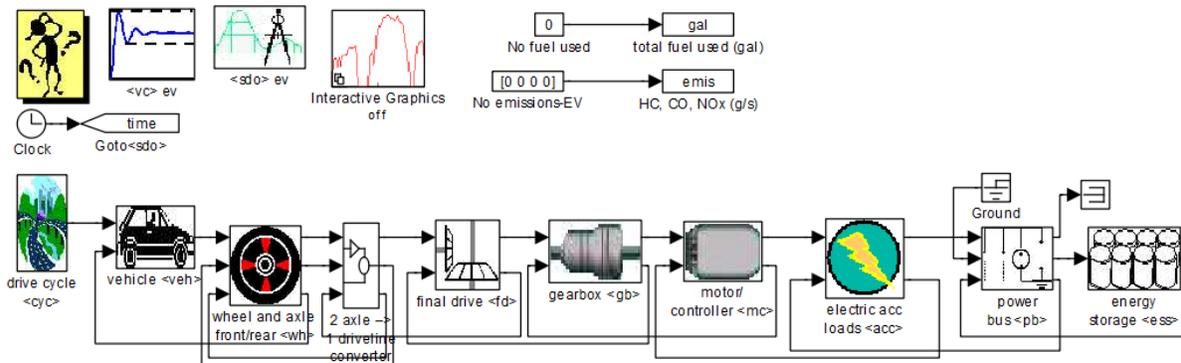
Figure 2. The model of an electric vehicle powered by a li-ion battery pack.
