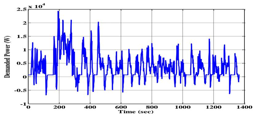
Figure 9. Demanded power for UDDS driving cycle
