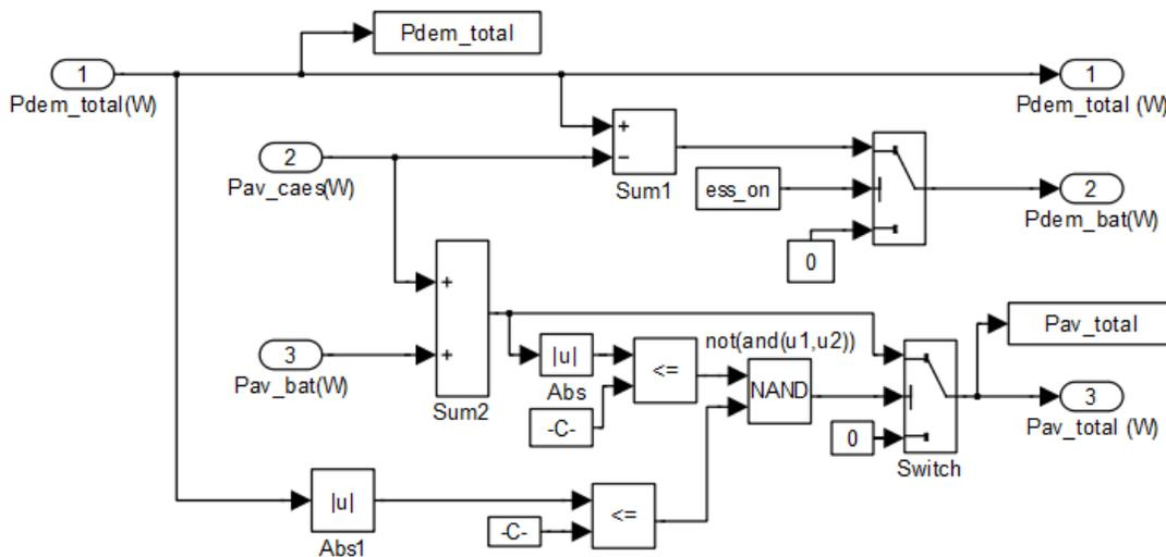
Figure 4. Simulink model of the power bus block
