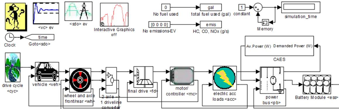
Figure 3. The model of an electric vehicle powered by hybrid energy sources
