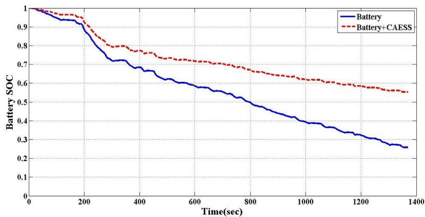
Figure 10. Changes in the battery SOC value for UDDS urban driving
