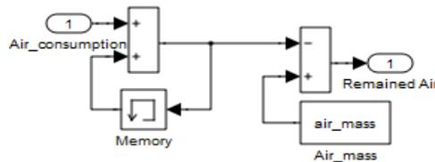
Figure 7. Simulink model of the air tank
