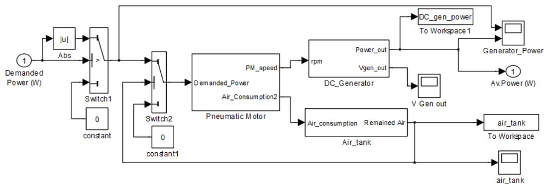
Figure 5. Simulink model of the CAES system
