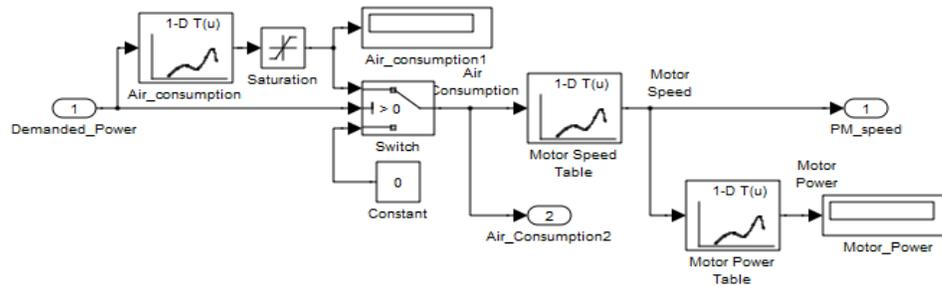
Figure 6. Simulink model of the pneumatic motor
