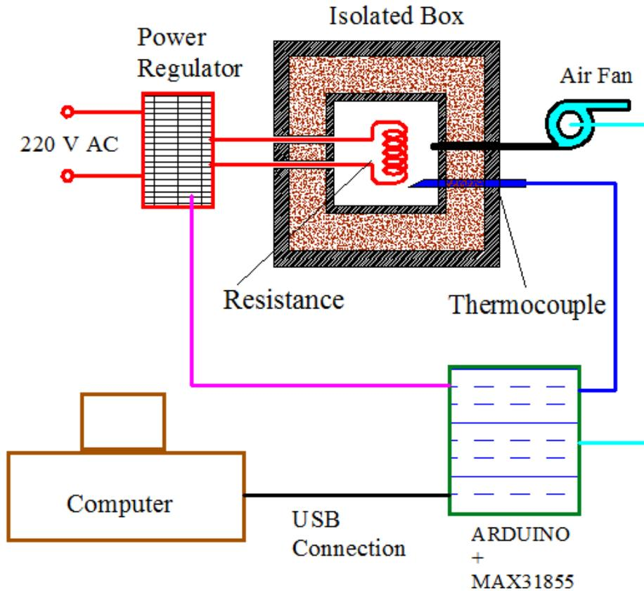
**Figure 1.** The scheme of temperature controlled heating system
