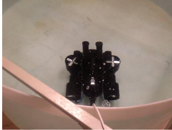
Fig.10. Horizontal control tests by the terminal
