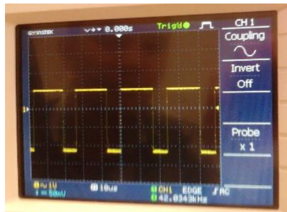
Fig.6. %70 PWM Rate from PA0 port which drives the M1.
