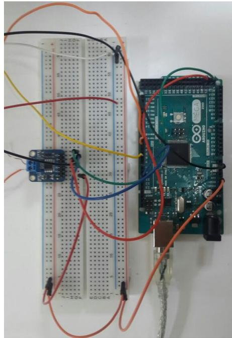
Figure 3. Arduino MEGA 2560 and MAX31855 Amplifier
