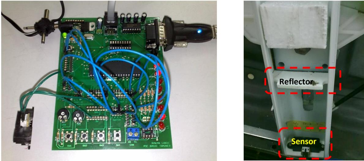
Figure 2.5: GP2D12 tested on the PIC board and power window regulator
