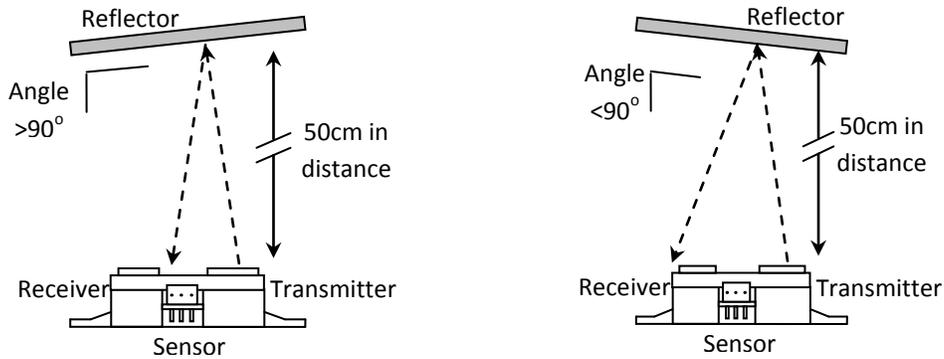
Figure 4.0: Reflector’s illustration due to manual fabrication on the reflector’s track in a farthest distance
