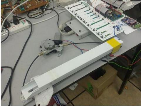
Figure 3.0: Overview of Kaptoris DAQ system and power window regulator
