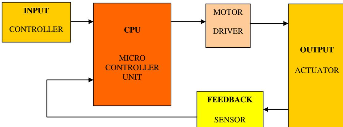
Figure 2.8: Integrated control system block diagram
