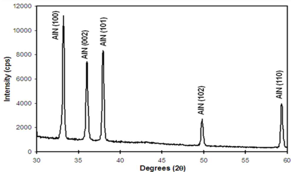
**Figure 3.** XRD pattern of the AlN nanostructures indicating hexagonal wurtzite structure.
