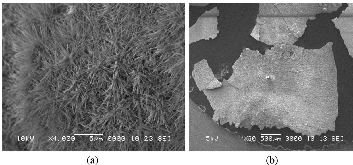
**Figure 2.** SEM images of catalyst-free grown ultra-dense AlN nanostructure films at 1100°C: (a) high magnification (AlN nanorods with 30 nm tip diameter and ~10 μm length); (b) low magnification films
