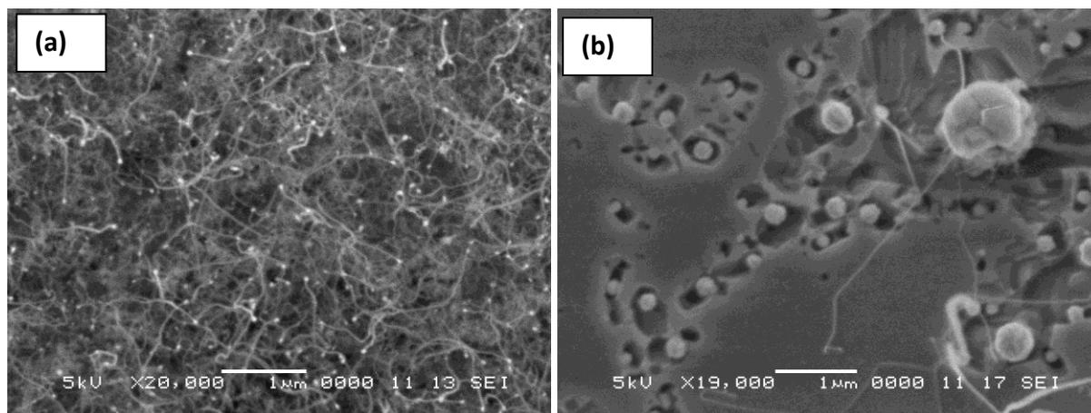
**Figure 1.** SEM images of AlN nanowires grown at 1100°C under H<sub>2</sub> with different catalysts: (a) Ni-film, (b) Co-nanoparticles solution.
