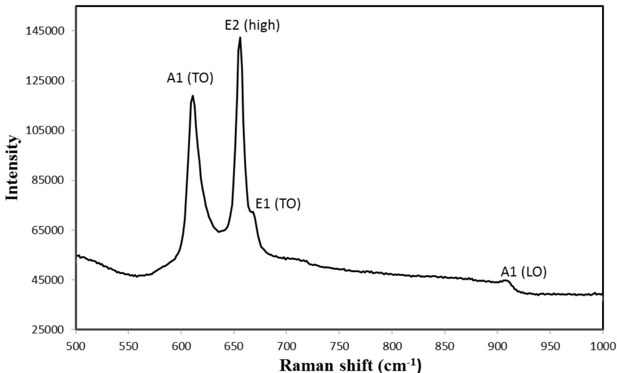
**Figure 4.** Raman spectrum of the AlN nanostructures.
