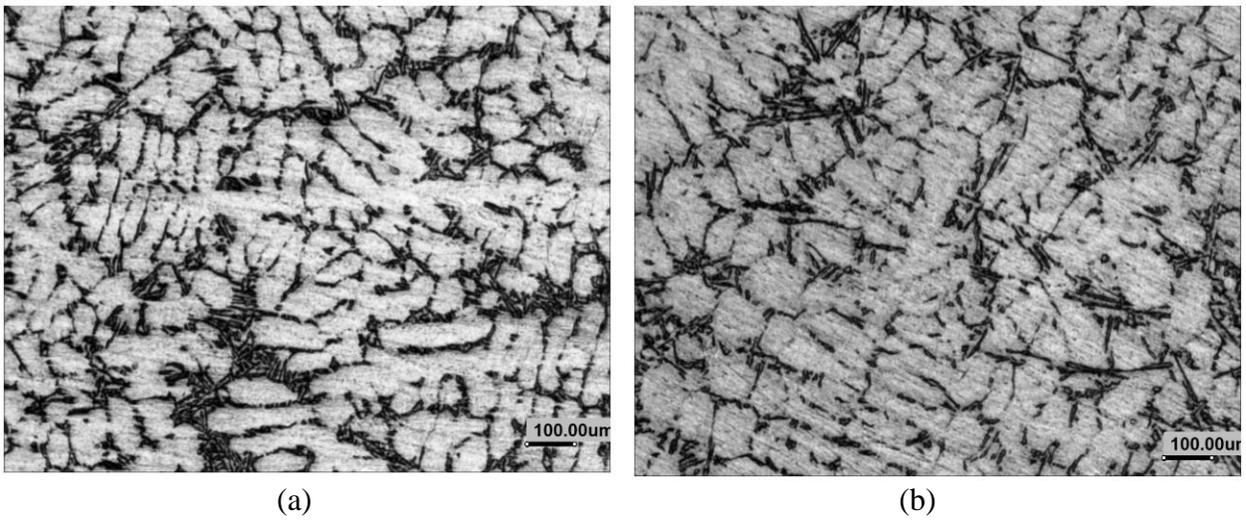
**Figure 6.** Microstructures of the  $AlB_3$  grain refined alloy
