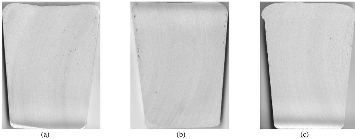
**Figure 3.** RPT samples produced from the degassed melt (a) as-received, (b) Sr modified, (c)  $AlB_3$  grain refined
