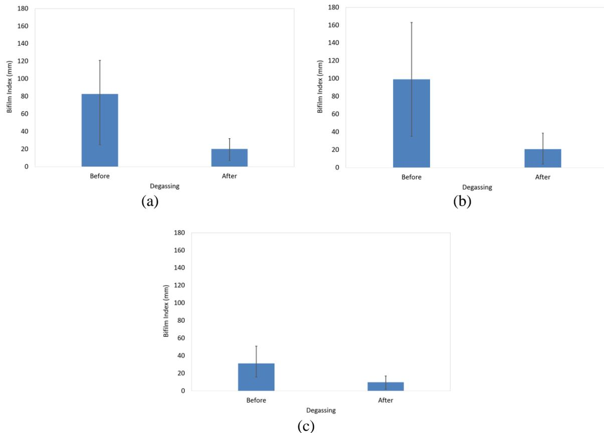
**Figure 7.** Bifilm index change of the melt before and after degassing
