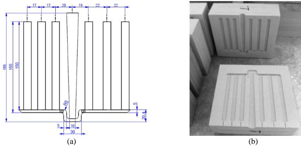
**Figure 1.** a) The dimension of the mould b) The sand mould used in the casting trials
