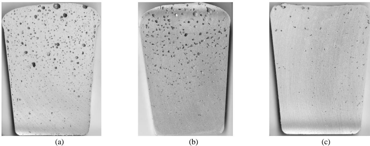
**Figure 2.** RPT samples produced from the untreated melt (a) as-received, (b) Sr modified, (c)  $AlB_3$  grain refined
