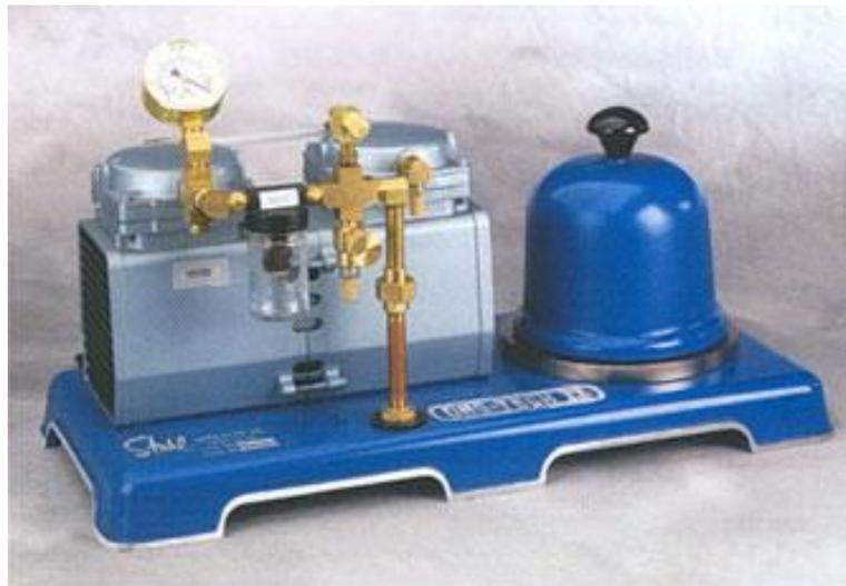
**Figure 4a.** Reduced pressure test machine
