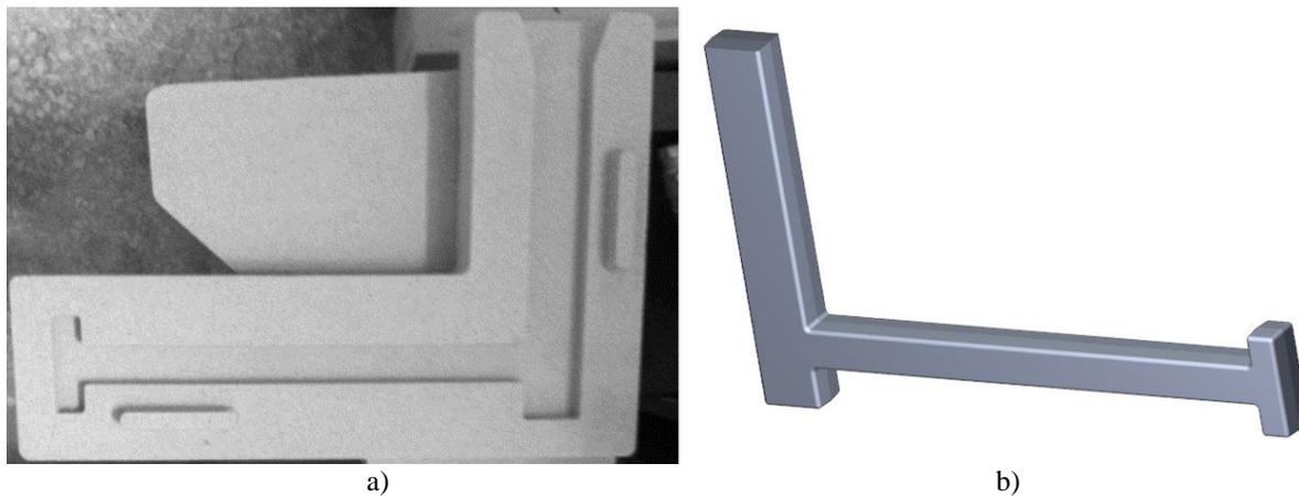
**Figure 1.** a) Sand mould used in the castings, b) dimension of the cast part that is produced
