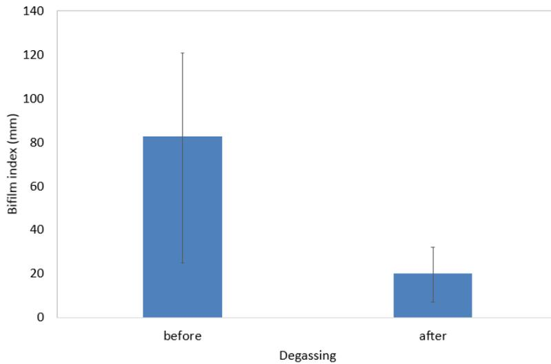
**Figure5.** Bifilm index measurements
