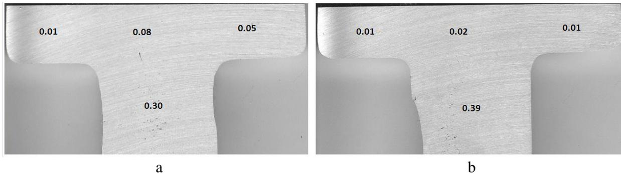
**Figure 7.** Distribution of pores along the sectioned areas of the cast part
