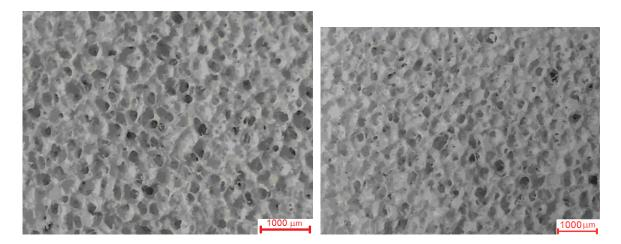
Figure 6. The ceramic foams produced at a) 1200°C b) 1250°C
