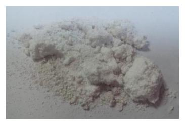
Figure 4. The collapsed HA foam produced from spray dried powder after sintering
