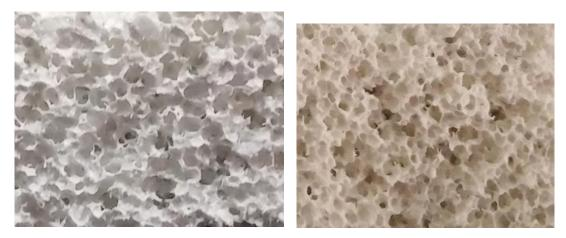
Figure 3. The reticulated structures of HAp prepared from a) finer powder b) coarser powder
