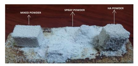
Figure 5. Preforms produced using different powder morphologies
