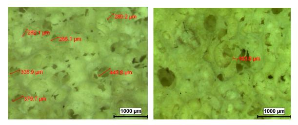
Figure 9. Pore size and arm thickness in the HA samples with 10% bentonite
