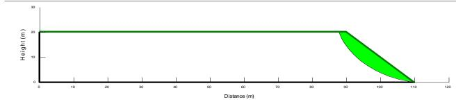
Figure 3. Slope geometry and failure surface obtained for a 20 m high slope.
