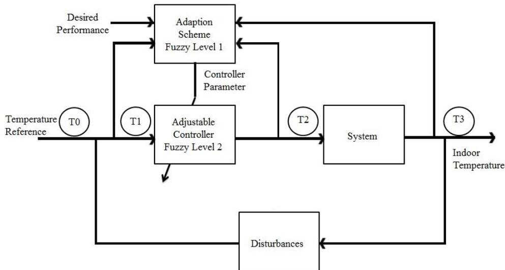
Figure 2: Controller Scheme
