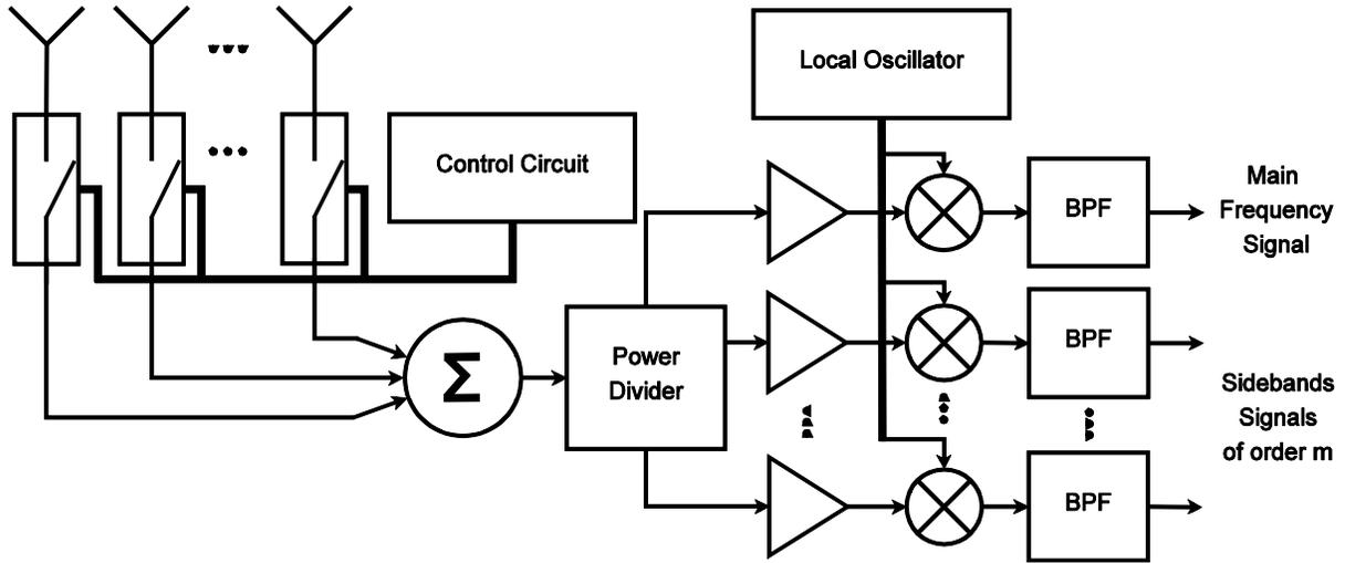
**Figure 1.** Block diagram of potential receiver structure for a time-modulated linear array
