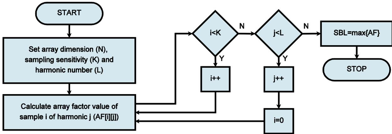
Figure 2. Flow chart of maximum sideband level calculation for a single harmonic frequency with conventional method
